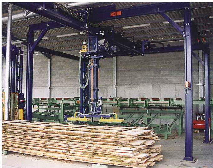
Movimentatore a depressione per tavole singole. Vacuum handling systems for single boards.
